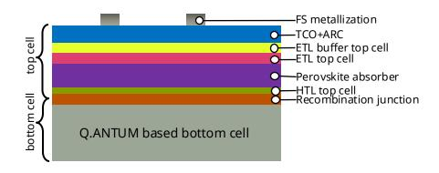
2-Terminal Perovskite-on-Silicon to overcome practical limit of silicon solar cells Qcells' next gen Q.ANTUM technology based on tandem has efficiency headroom > 30%
