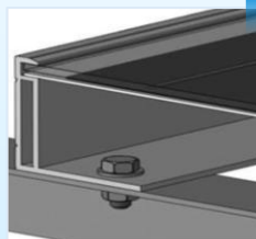
Figure 1. PV module installed with bolt fitting method.
