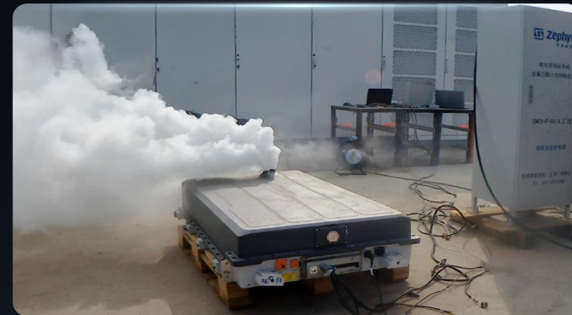
Pack thermal runaway jetting test
