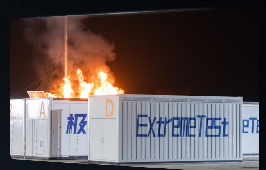
20MWh large-scale burning test
