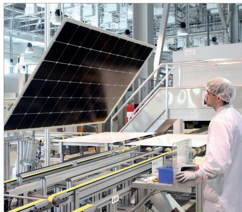
Figure 6. Visual control station on Hevel's production line.
