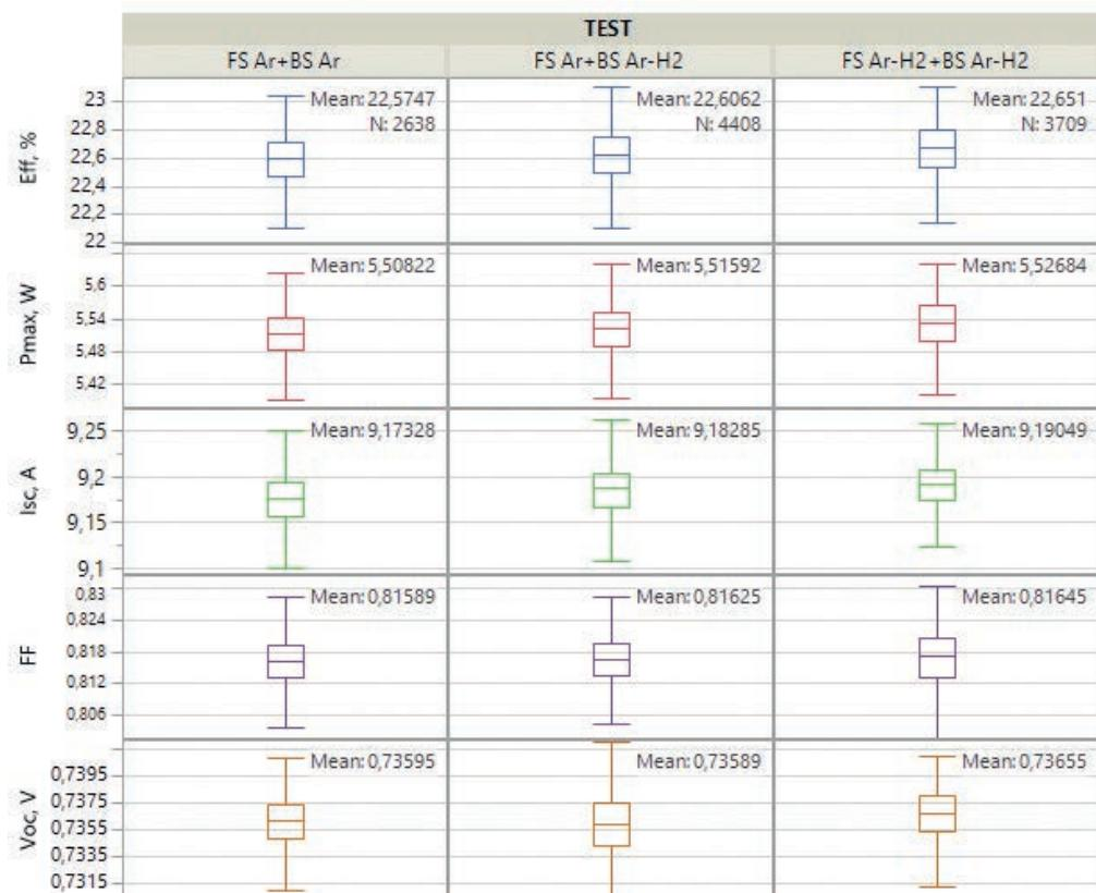
**Figure 4.** Results of ITO layer optimization by adding an Ar/H<sub>2</sub> mixture during magnetron sputtering.
