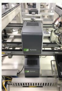
Example: inline bifacial cell measurement
