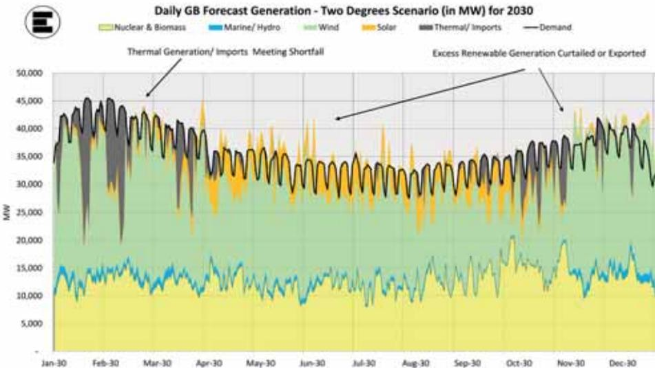
Figure 2. EnAppSys’s generation forecast for Britain in 2030 under National Grid’s 2 Degree Future Energy Scenario
