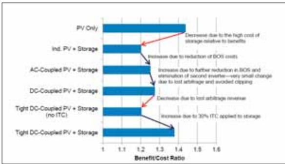
**Figure 2. Benefit/cost ratio for different PV-storage combinations [1]**
