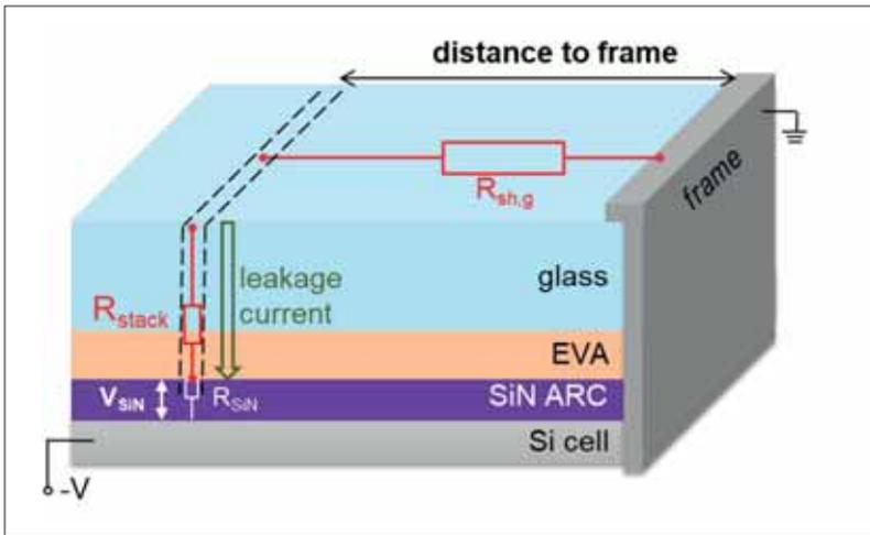
**Figure 1. Equivalent circuit for the leakage current path at the front side of a framed PV module (voltage divider model).  $R_{sh,g}$  and  $R_{stack}$  are subject to changes due to environmental influences like soiling and moisture. The voltage across the SiN ARC of the solar cells determines the strength and rate of PID and depends only on the local leakage current (density) through the encapsulating layer stack and the electric properties of the SiN layer ( $R_{SiN}$ )**
