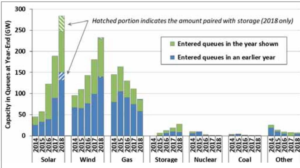
**Figure 10. Solar and other resource capacity in 37 selected interconnection queues across the US**
