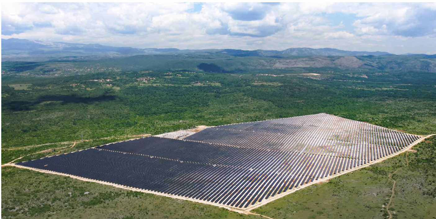
Figure 15. Large utility-scale system in Bosnia and Herzegovina using bifacial AIKO modules [17]
