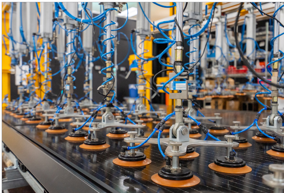
Figure 5. Dynamic mechanical load testing at RETC, part of the VDE Group
