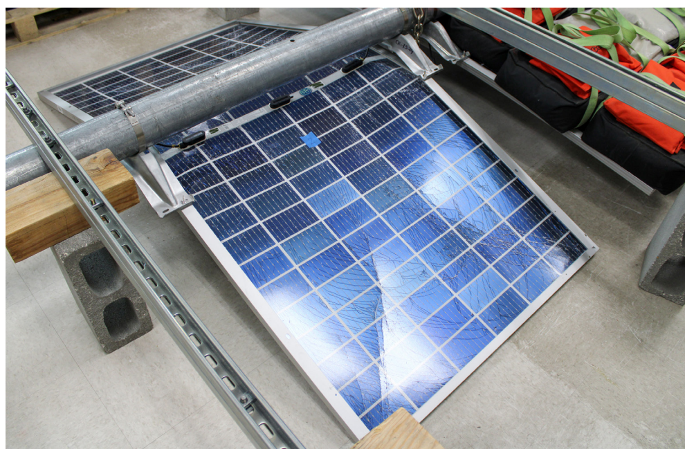
Figure 4. Catastrophic failure resulting from mechanical load testing
